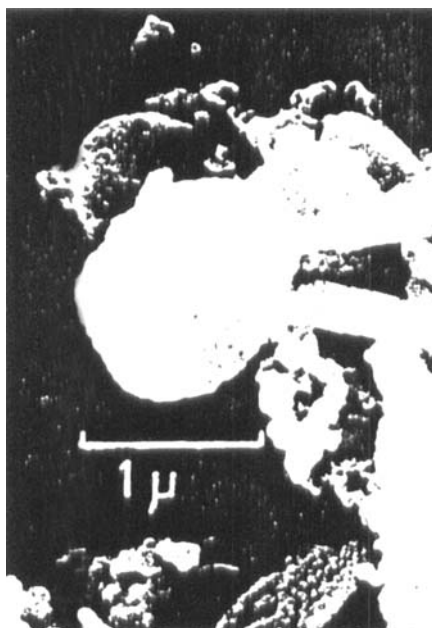
FIG. 7. Surface view of polymerized system. Polymerization of MMA ( 3 \text{ cm}^3 ) was carried out in water ( 5 \text{ cm}^3 ) containing 0.1 g of PSS-Na (No. 4) at 85^\circ\text{C} for 3 hr on standing. The water layer was pipetted out and diluted with water to 500 \text{ cm}^3 .
